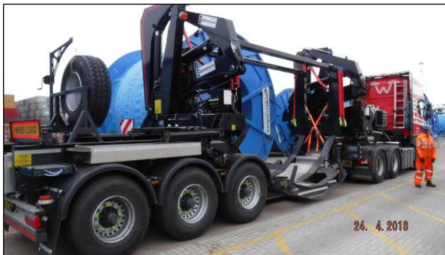
Plate 6 - Photo of Cable Drum Delivery Vehicle
